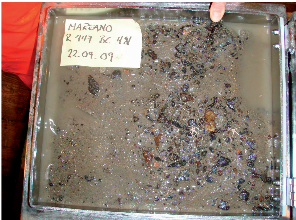
Figure 4. The box corer gives us a virtually undisturbed sample of the seabed but it is difficult to use on a rocky bottom. The image shows a gravelly surface where the box corer has closed nicely further down in the sediment.
