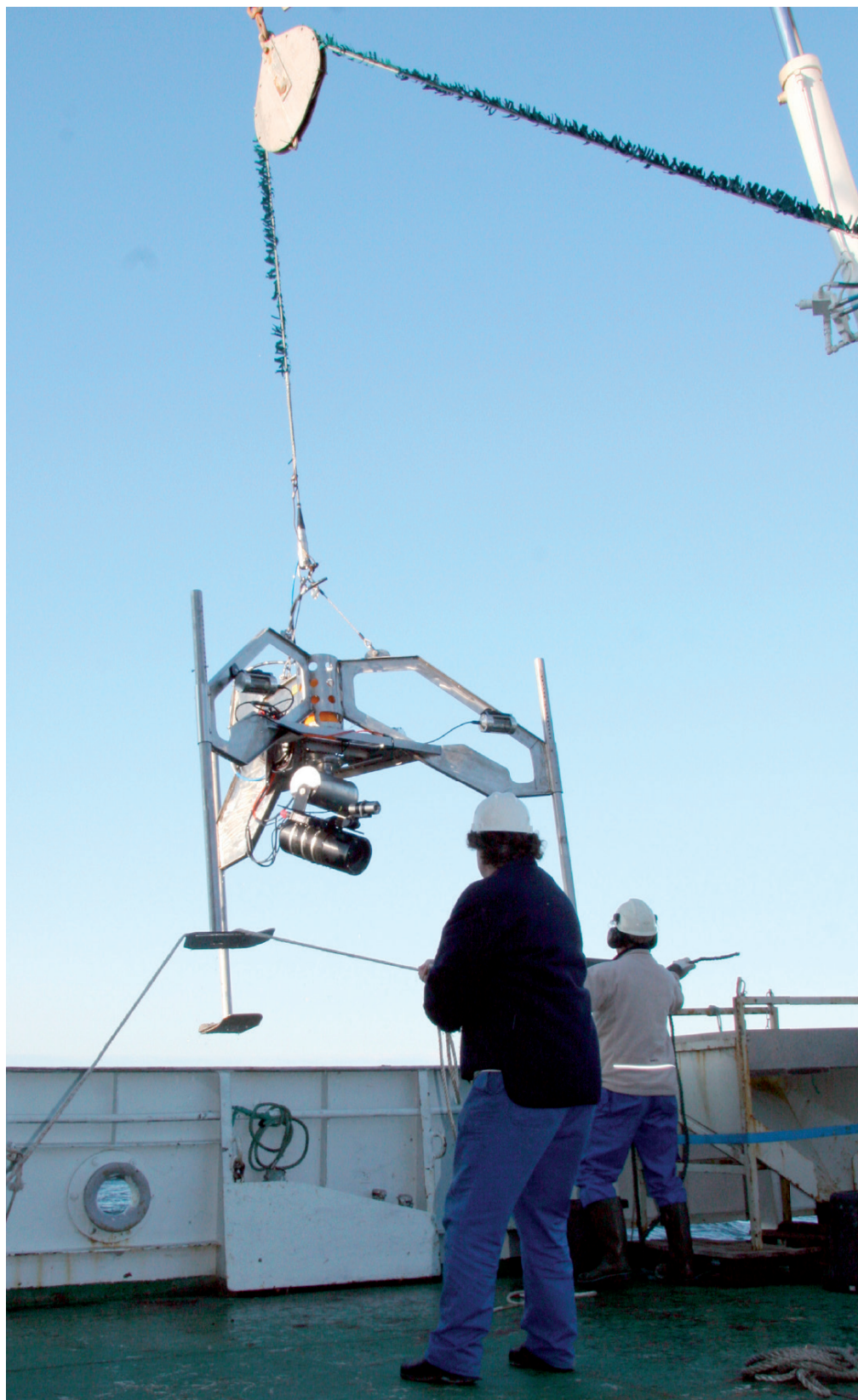
Figure 3. The video rig, Campod, is an important tool in MAREANO. It can record down to 6000 metres. It is lowered down on the seabed where it can zoom in on details - it is also towed slowly over the bottom, ensuring that details are not blurred. In addition to two video cameras, the Campod is equipped with a depth gauge, and a laser scale, as well as sensors to measure temperature, particle content, current and height above the seabed. In order to know where the rig is at all times, it is equipped with a so-called transponder that sends information back to the ship about its position and depth.
