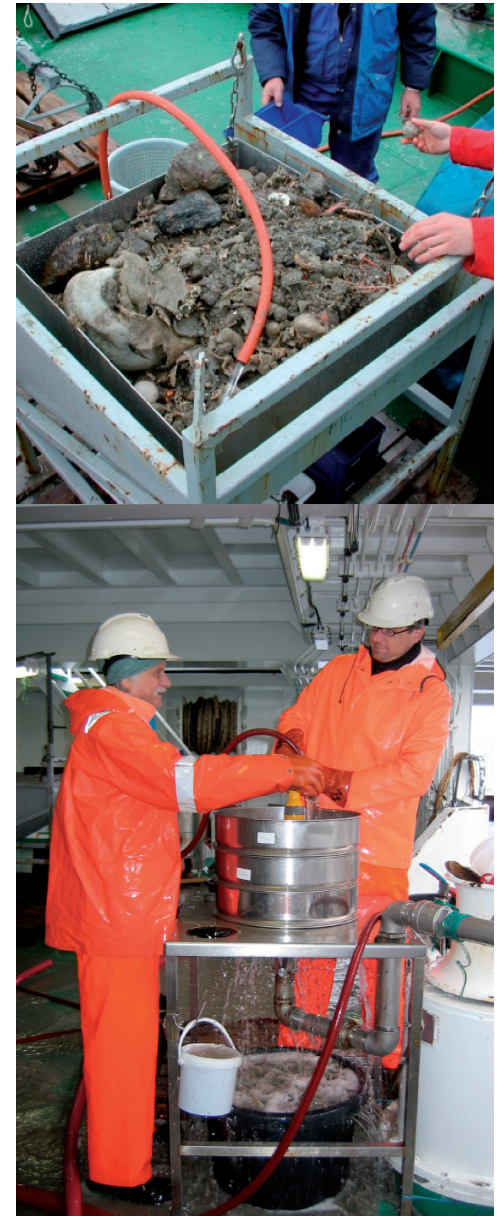
Figure 5. Sieving removes most of the sediments from the samples and simplifies the sample collection considerably. The beam trawl is meant to capture the large fauna living on the seabed and just under the surface but on a soft bottom it sometimes digs into the seabed, bringing back large amounts of clay and silt. Everything is then sieved through coarse and fine meshes before the samples are put in formaldehyde. The sieve, in the lower picture, is used for grab samples. The content is retained as several size fractions by the sieves.
